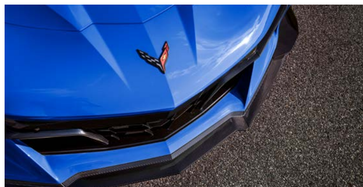
The front section was developed to optimise the cooling requirements of the Z06.
