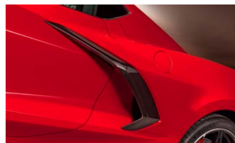
The door handles and the tailgate and bonnet release mechanisms have been concealed.
