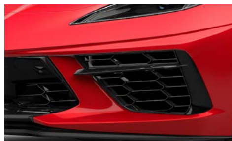
Air intakes under the engine compartment of the convertible.
