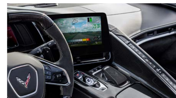
Performance Data Recorder for analysing racetrack laps
